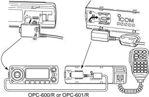
A ferrite core is adapted for the USA version.
