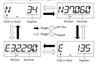
⑧After checking the current position, push any key below the display to return to normal operating mode.
